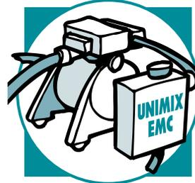
A way to get very accurate mixing of cleaners is to use a positive displacement proportioning pump such as the XYBEX UNIMIX.<sup>™</sup> Its big advantage is its high accuracy which is unaffected by changes in water pressure, flow rate, or the liquid level in the barrel. On the other hand, a UNIMIX carries a higher price than a venturi mixer, and it does have some moving parts.
