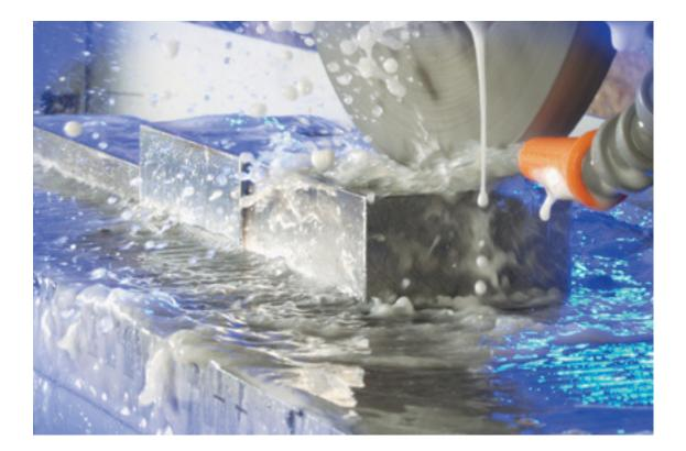
Figure 3. A TRIM<sup>®</sup> C320 being used to surface grind. Coolant management is especially important in grinding, where the fluid is quickly contaminated with the grinding swarf.
