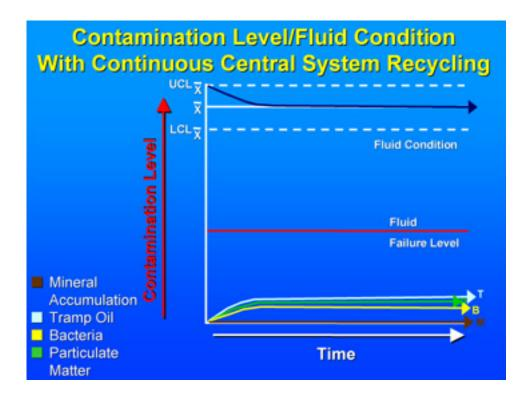
Graph 3. Contamination level with continuous central system recycling.
