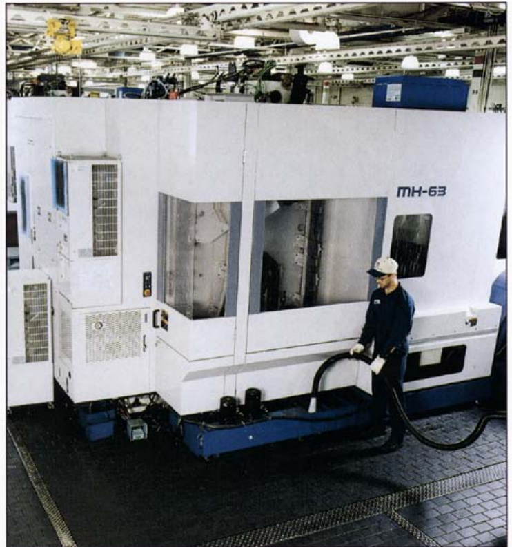
Technician cleans the sump of a Mori-Seiki machining center. Easy access to the sump makes it more likely that regular maintenance will be performed.
