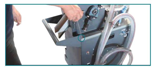
Unscrew the two screws, one left and one right beside the magnetic separator.
