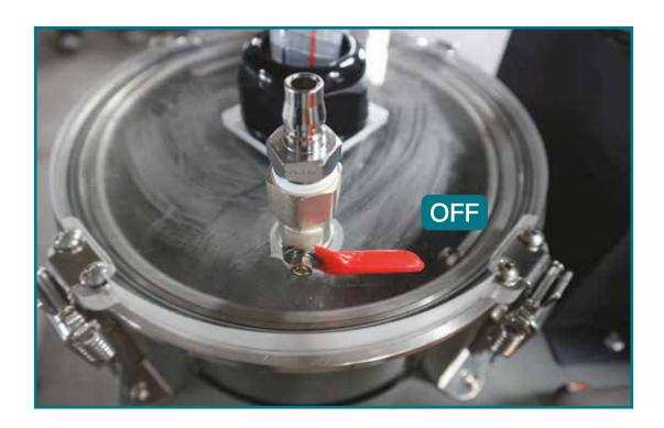
Switch the air pressure relief valve off when the maintenance is finished. Now it's ready for the next coolant tank cleaning task.
