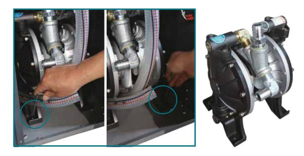
Remove the two screws fixed at the base and now you can replace the air pump.
