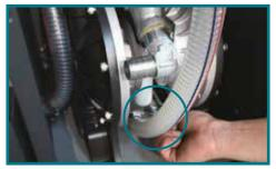
Before you disconnect the pipelines, do note and remember how they were originally installed to avoid re-installing confusion. The air pump is connected to total 4 pipes, 2 for inlet and 2 for outlet. Loosen all hose clamps and disconnect all the pipelines.
