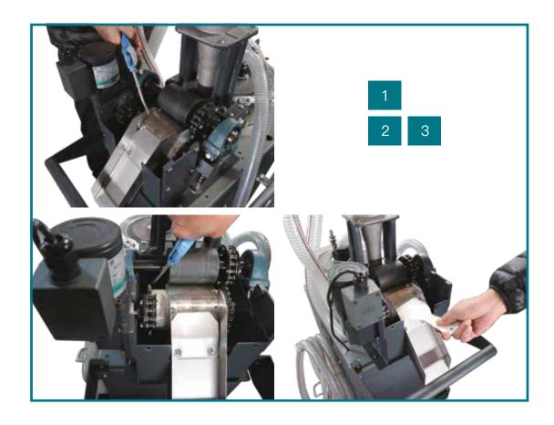
Use the scraper to remove the sludge on the discharge portal, and then use the equipped air gun to clean up all the possible particulates around the separator. Be sure there is no clogging or accumulation.
