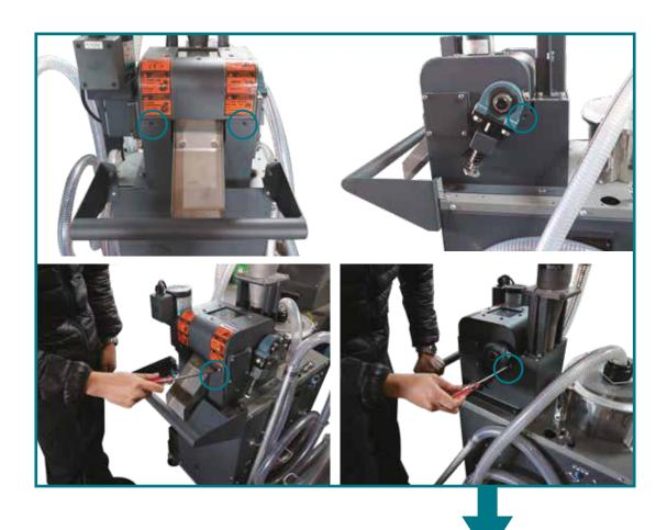
Loosen all 4 screws (2 at the front and one at each side) in order to open up the cover of the separator.
