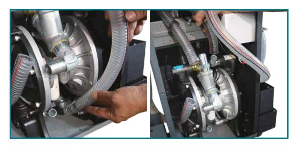
**STEP 6**Pipelines disconnected as shown in the above pictures.
