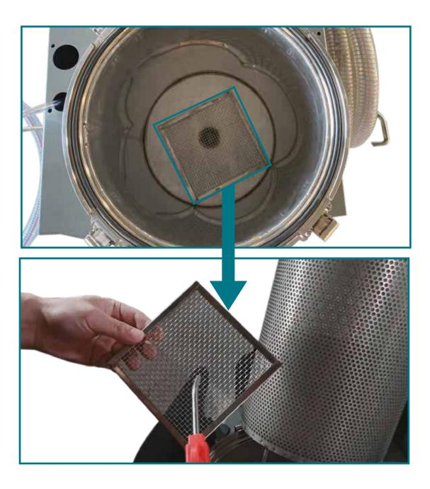
There's a rectangular mesh underneath the filter. Clean this mesh regularly with the air gun or water as well.
