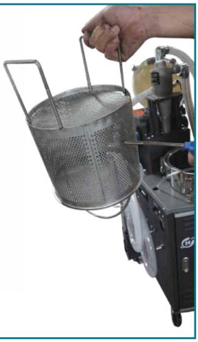
Hold the filter upside down and use the air gun or water to blow/clean the remaining impurities.
