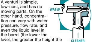
cleaner solution can get more lean). And, if the viscosity of your cleaner is affected by temperature, a cold barrel can give you a leaner solution than if the cleaner were at room temperature. (So, if you store your drums outside in cold weather, it's a good idea to bring them inside for a day or two to warm up before you need to use them.) Don't get us wrong, venturi mixers are still a good choice to mix cleaners accurately for a
