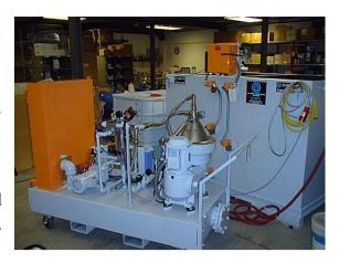
The unit is equipped for use on high temperature and high pH fluids. And being mobile, it is able to process fluids in different locations within the Sunderland factory. With a flow rate of 750-1400 litres per hour dependant on the type of fluid used, the XYBEX® removes both free and emulsified tramp oil to 0.5% or less and particles down to 8 micron or less.
