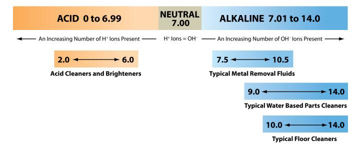
The following chart shows the approximate pH of some common materials and the pH value of some typical MWF formulations and components. These numbers are offered for reference only, not to be used as specifications, etc.
