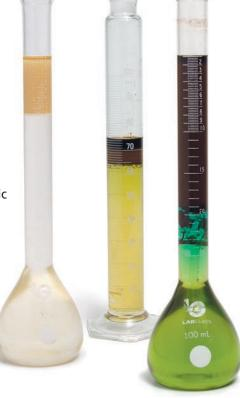
The nature of this test is quite subjective and relies a good deal on operator technique. The process gives very good and repeatable results but does take six to 18 hours between sample grab and result. The method also provides additional and potentially very useful information, e.g. tramp oil levels, concentration by product oil, and concentration by surfactant content.
